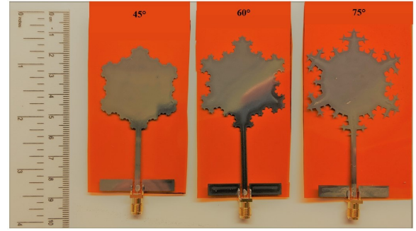
Figure 7: Design of three transformed Koch snowflakes for 45°, 60°, and 75°
